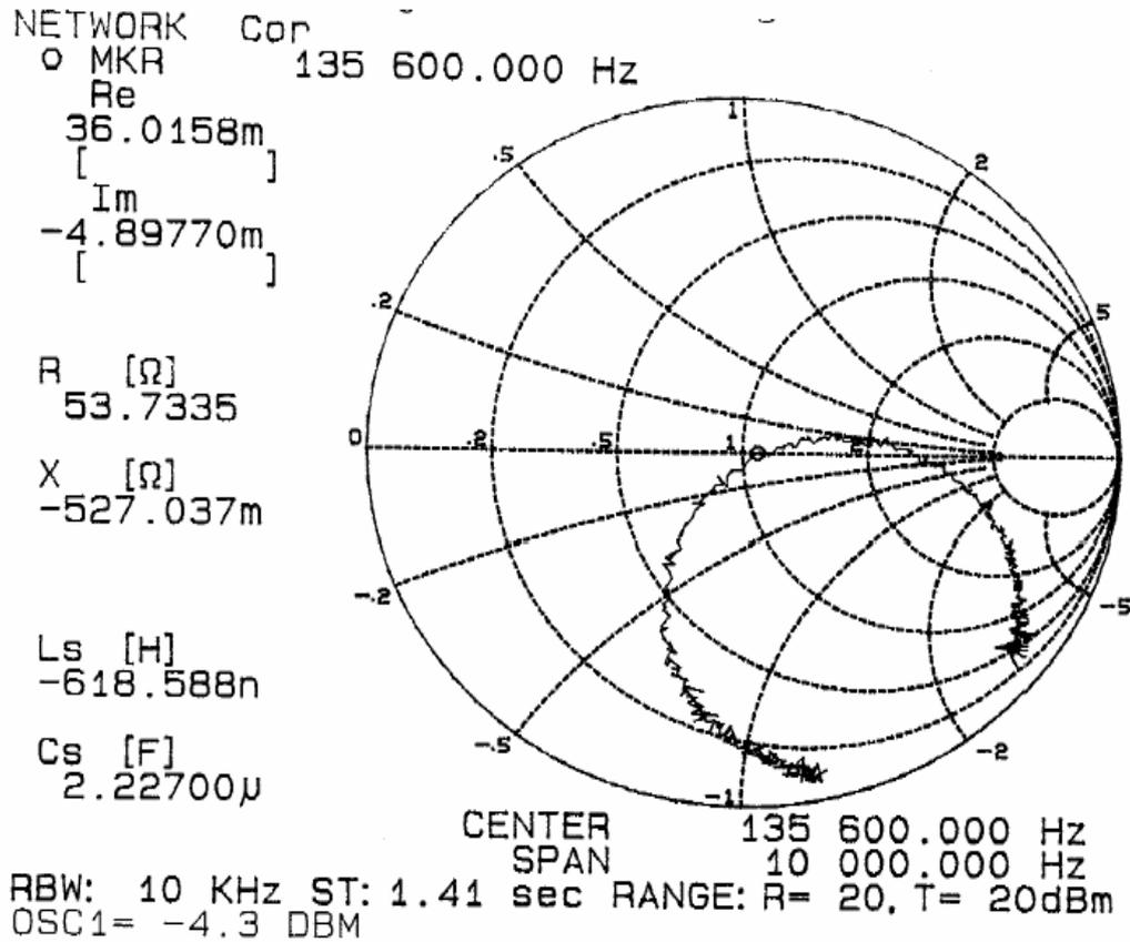
5.0 Measured values of antenna impedances for 540 kHz +/- 20 kHz
